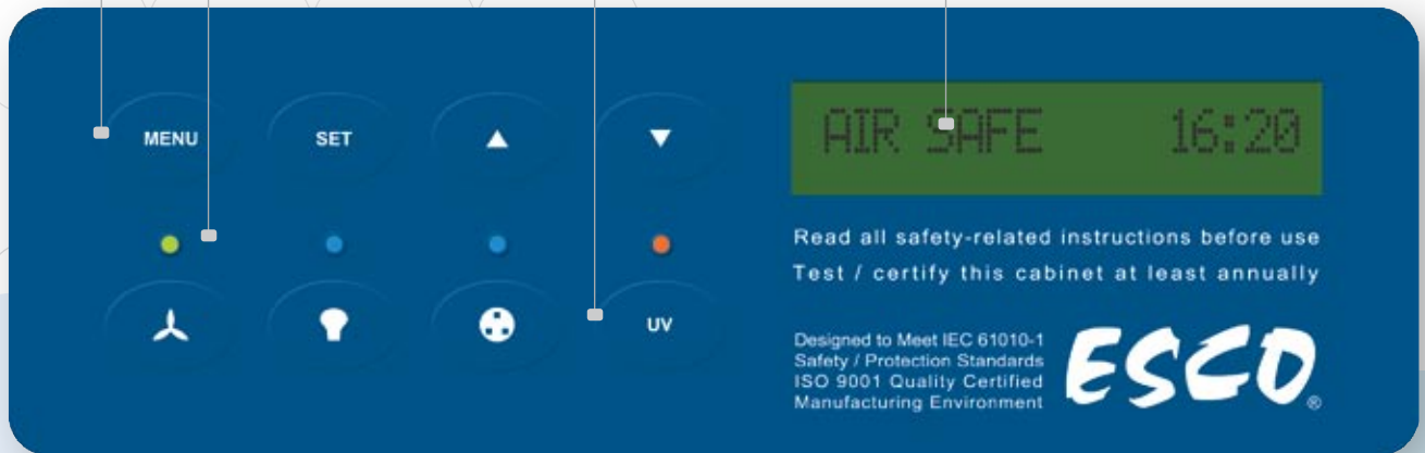
Sentinel Microprocessor Control System, Programmable
